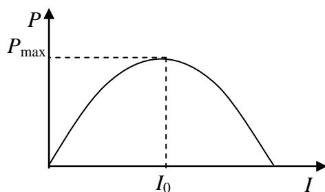
If the current varies in a sufficiently large interval a maximum power  $P_{\max}$  can be detected at a certain value,  $I_0$ , of  $I$ . Theoretically, the  $P(I)$  dependence is given by:
