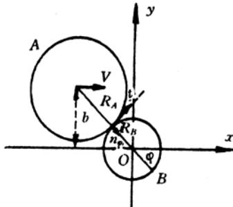
During the collision at the point of contact A and B acquires the same tangential velocities, so we have
