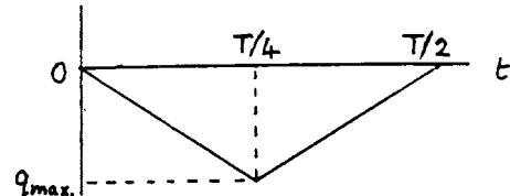
5) This question can be discussed without making a full circuit analysis. One only needs to realize that the rate of flow of charge into the amplifier is divided into a rate of charging of the capacitor,  $C dV/dt$ , and a conduction current,  $V/R$ , through the resistor. There are then two extreme situations, depending on whether the amount of charge lost by leakage during one quarter-period is small or large compared to  $CV$ .
