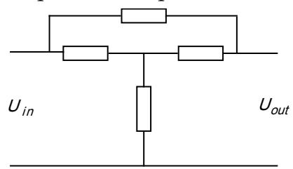
At frequency  $f_0$  the phase lag between the two voltages is zero.
