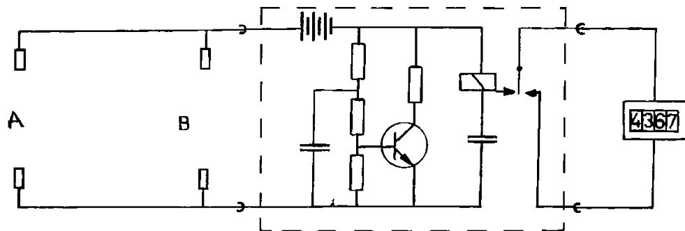
The purpose of the transistor circuit is to keep the relay position after closing of the contact at B, even if this contact is opened afterwards for a few milliseconds by a jump or chatter of the cylinder.
